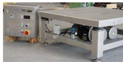
SRF and vibrating table made of stainless steel
